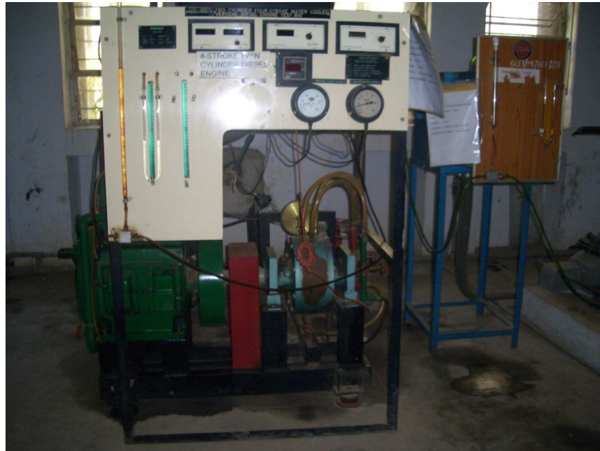
Four stroke, twin cylinder C.I. engine set up with an hydraulic dynamometer
