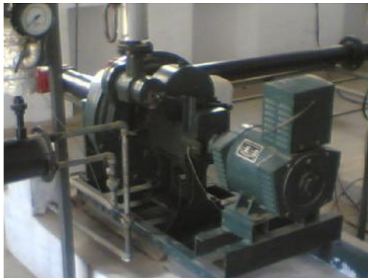
Single stage, velocity compounded impulse turbine
