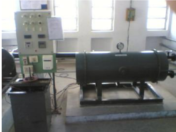
2 pass shell & tube condenser with water rheostat
